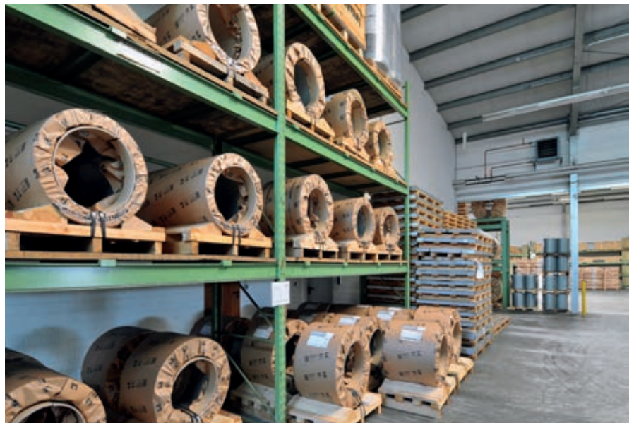
Storage of coils with wooden sleepers
